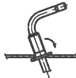
3. Put seal, washer and tighten nut.
